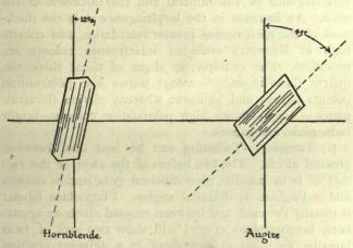
Fig. 44.—Hornblende: Extinction Angle, 12°. Augite: Extinction Angle, 45°.
